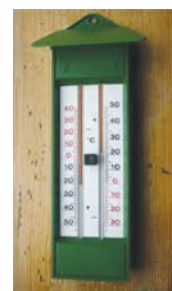
d. Maximum - minimum thermometer
